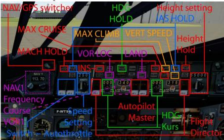
All the switches you need are listed here. The co-pilot will tell you when to operate switches and make adjustments.
