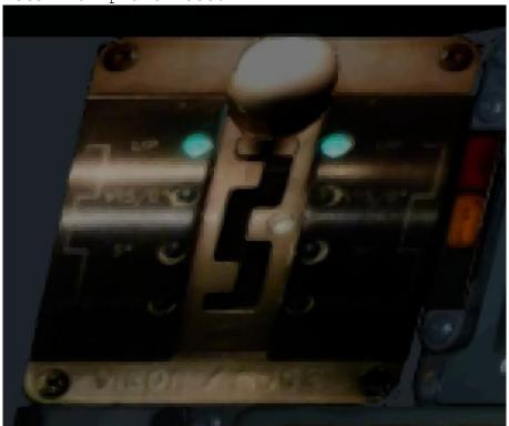
The nose of the plane is lowered with this lever. A combination of right and left click with the mouse (r,r,l,l,r,r,l) for complete lowering).
