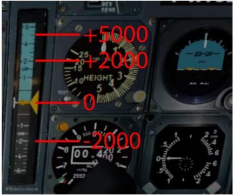
The Concorde climbs normally with 5000ft/min. Below 10000 feet, however, only 2000ft/min. The sink rate is always 2000ft/min.
