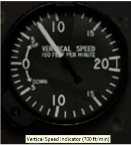
A deviation of approx. 70Ft/min (at a climb/descent rate of 500Ft/min) does not play a role in normal flight operations, which is probably why the error was never corrected. In the "helicopter school", however, more precise adherence to speed, altitude and climb rate is required than in normal flight operations.
