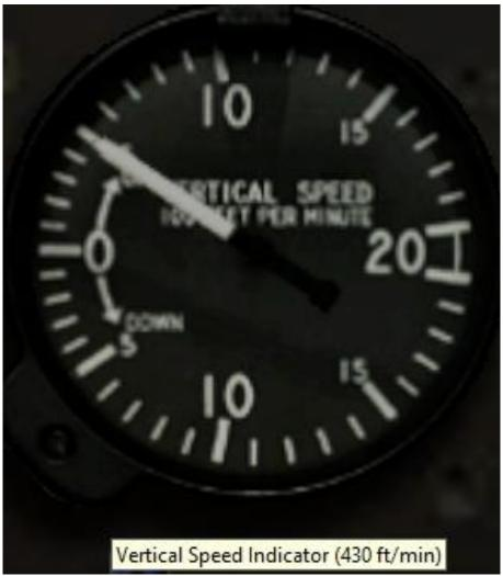
Display at actual climb rate: 300Ft/min 500Ft/min 700Ft/min
