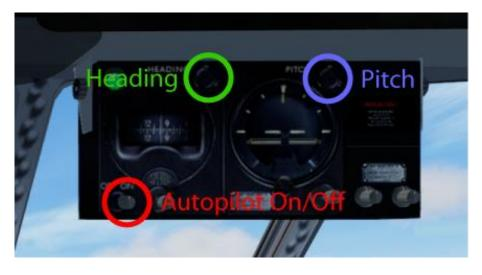
Autopilot On/Off: Activates heading and pitch. Heading (HDG): is as usual, set heading 100 and you fly in that direction. Pitch: This is the replacement for Climb Rate. You want to climb to 10000 feet at 1000 feet/min. Set Pitch to about 9, then you will reach about this climb rate. Depending on the power you have to readjust and when you reach 10000ft, reduce power and readjust pitch in the autopilot (probably set it down to +2 to 0).
