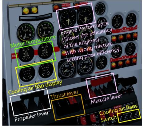
Here you can adjust thrust, propeller speed, mixture, cooling air flaps and monitor temperatures.
